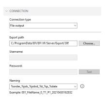
When set up this way, the Fiery XF server RIPs the job and creates a \*.bco file. Use the printer software to select the \*.bco file and print the job. For more information on how to use the printer software, see the Pro 30f Operator's Guide.
